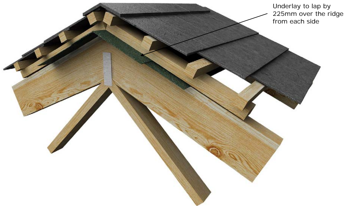
Figure 5: Sealed cold roof ridge detail
